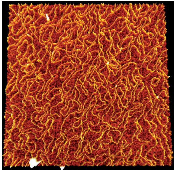
Figure 3. Three-dimensional topography image of pUC plasmid DNA adsorbed onto a mica substrate. The individual DNA strands are clearly visible against the mica background. Images were acquired on a BioScope Catalyst AFM operated in PeakForce Tapping in buffer solution using ScanAsyst Fluid+ AFM probes ( $k \sim 0.7\text{N/m}$ ). Image XY-Scale = 2μm.
