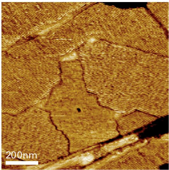
Figure 2. A 1μm Phase Image of a C<sub>60</sub>H<sub>122</sub> alkane. The C<sub>60</sub>H<sub>122</sub> is spincoated onto an HOPG substrate with the resulting ultra-thin alkane layer exhibiting a lamellar structure ~7.5nm in width and ~0.4nm in height. Images were acquired on a BioScope Catalyst AFM operated in TappingMode using FESP AFM probes ( $k \sim 3\text{N/m}$ ).
