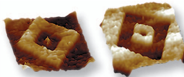
Figure 6. CFM scan of well-defined regions that terminate in either methyl or carboxylic acid groups. When a carboxylic acid-terminated tip is used for imaging (left), the carboxylic acid-terminated regions exhibit greater frictional force (lighter color) than the methyl-terminated regions. When a methylterminated tip is used (right), the friction contrast is reversed. No differences are revealed by the topographic AFM scan (not shown) since the functional groups are structurally quite similar. 50µm images acquired using the Digital Instruments MultiMode AFM system. Image courtesy of Dr. C. Lieber, Harvard University.
