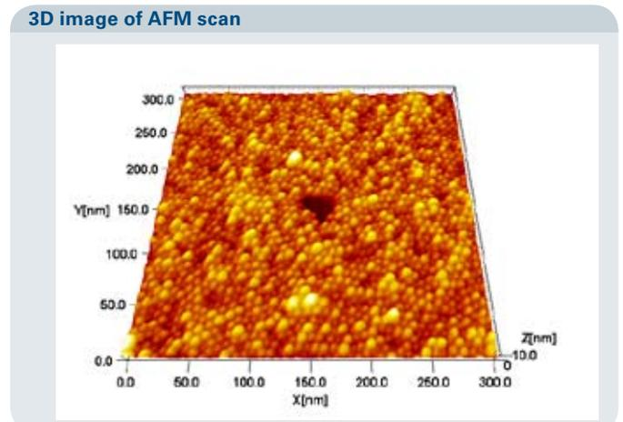
Fig. 3 3D representation of the 300 nm x 300 nm AFM scan. The spherical shape and close packing of particles is clearly visible.
