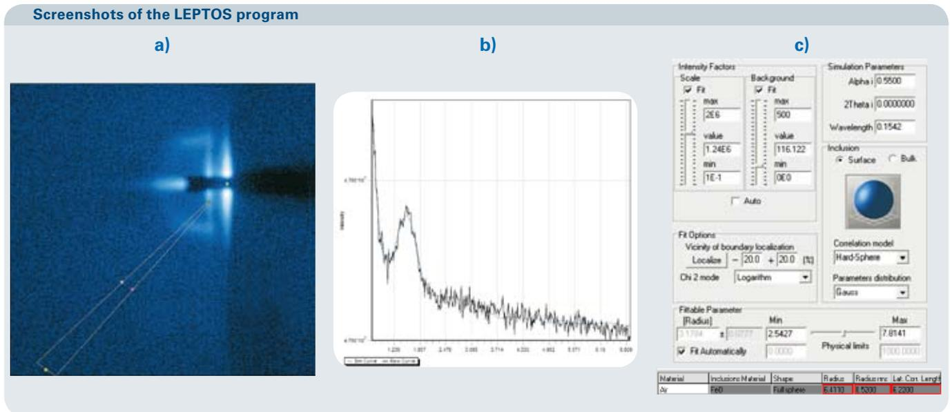
Fig. 6 a – c Left: a) 2D GISAXS map. b) Radial section from the map in a). c) Sample model used for the measurements
