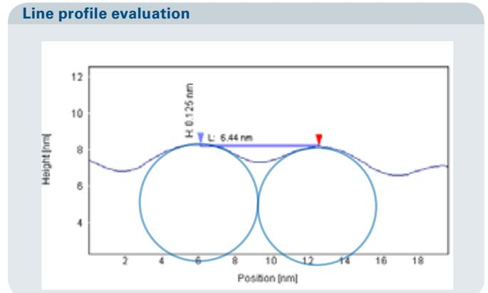
Fig. 2 Line profile from fig. 1 b). The blue circles indicate the spherical particles, the arrows the positions of maximum height (particle tops) used for size determination.
