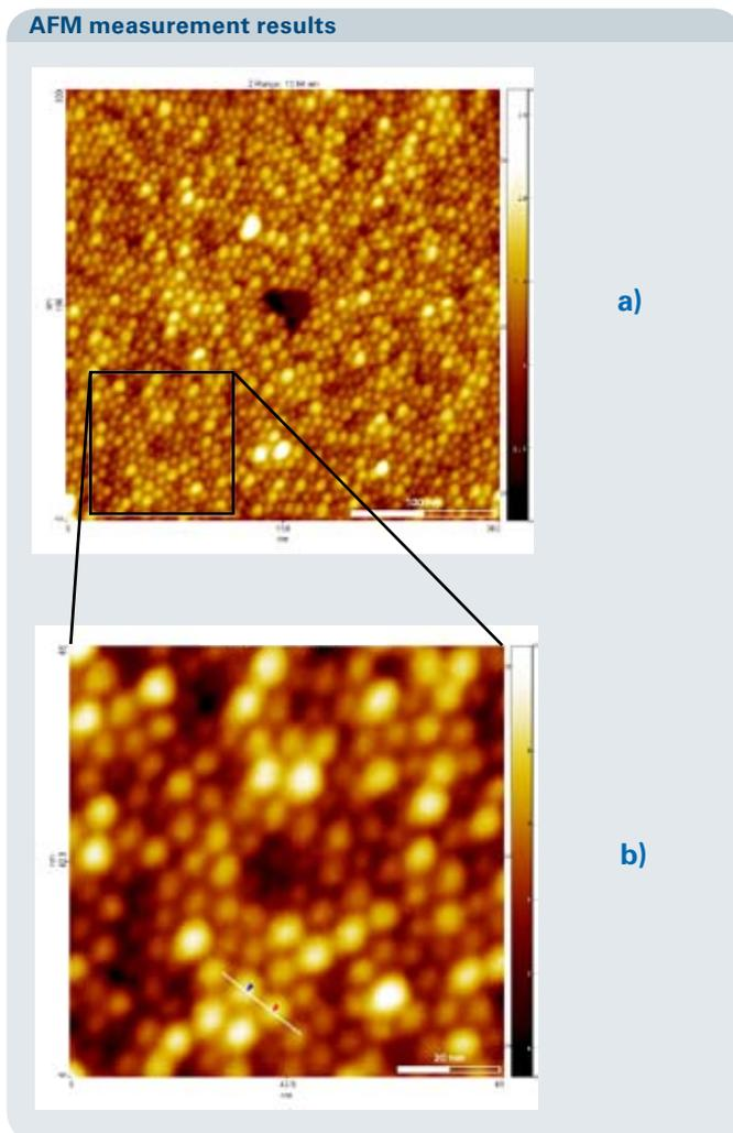
Fig. 1 a – b Top: a) 300 nm x 300 nm topography scan of FeO particle sample. Bottom: b) Zoom into a), scan size 85 nm x 85 nm. The white line with arrows indicates position of a line profile.
