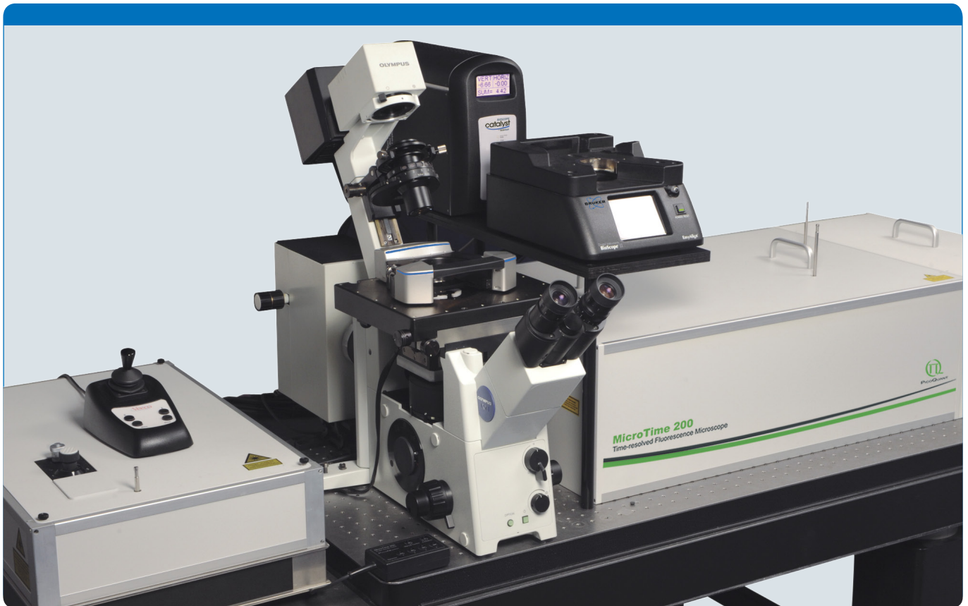
Figure 1. Combined setup of the BioScope Catalyst and the MicroTime 200. The AFM with its sample stage is mounted on the inverted microscope body of the MicroTime 200, which is configured for objective scanning.
