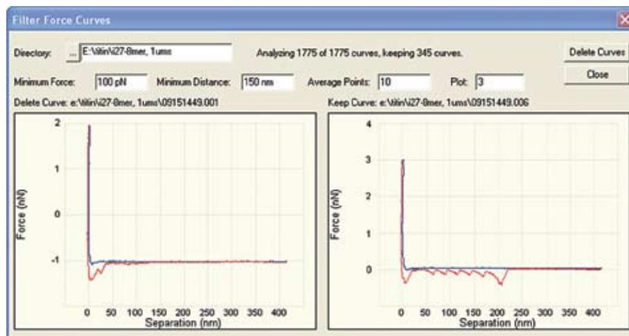
Figure 1: The Filter Curves view allows force-distance curves that contain no useful data to be rapidly identified and discarded according to user-defined criteria.
