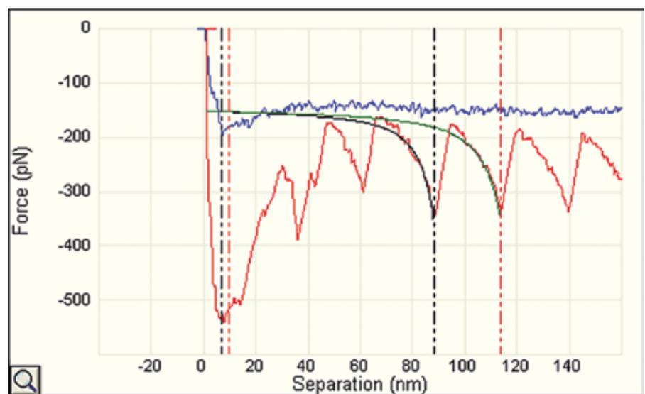
Figure 7: Worm-like chain fit of a titin extension curve
