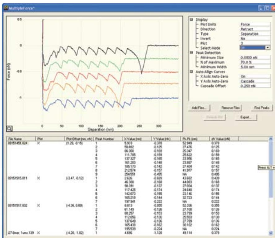
Figure 5: The Multiple Curve Analysis view can also display force curves in a “cascade” style view, which makes comparing several curves more convenient.
