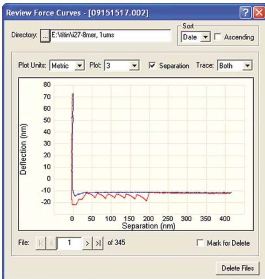
Figure 2: The Review Curves view allows the user to rapidly sort through force-distance curves without individually opening the files.
