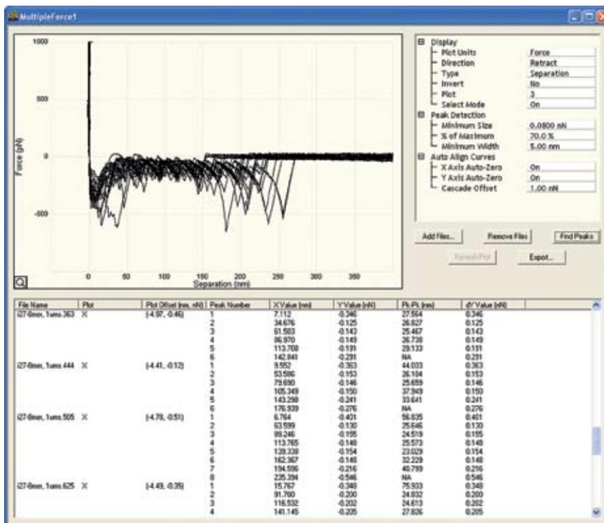
Figure 4: The Multiple Curve Analysis view offers functions that automatically align force curves by their contact points, finds adhesion peaks according to user-defined criteria, and can create a report of the tabulated peak forces and peak-to-peak distances.
