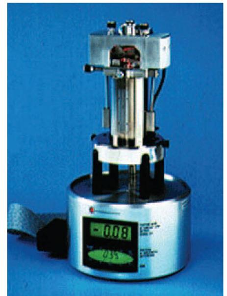
Figure 2. The MultiMode microscope includes an optical detection head, scanner, and microscope base. The compact, rigid construction of the microscope gives it the mechanical stability and low noise needed for high resolution. NEED NEW IMAGE...
