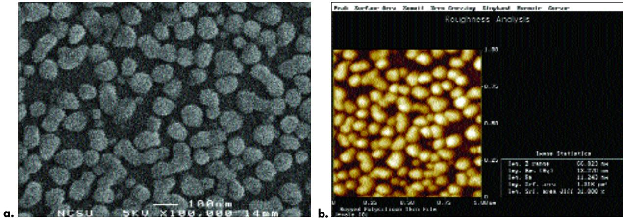
Figure 5. (a) SEM image of rugged polysilicon thin film. 100,000x, Bar = 0.1  $\mu\text{m}$ ; (b) TappingMode AFM image of the same with roughness measurement. 1  $\mu\text{m}$  scan.
