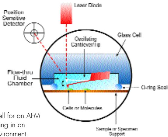
Figure 16. Fluid cell for an AFM which allows imaging in an enclosed, liquid environment.
