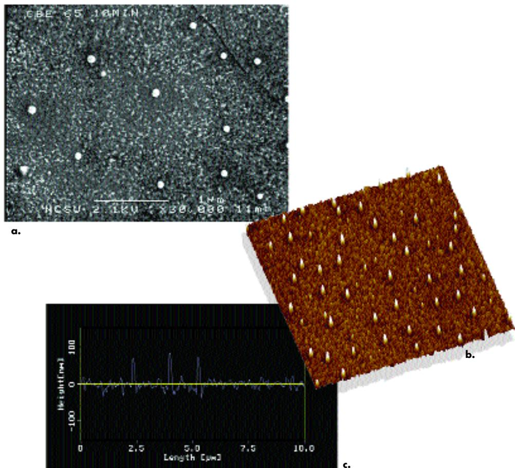
Figure 6. (a) SEM image of partially GaP-covered Si after chemical beam epitaxy deposition for 10 minutes. 30,000x, Bar = 1  $\mu\text{m}$ ; (b) AFM image of the same sample as in figure 6a showing the presence of nodules during the growth of GaP by chemical beam epitaxy. 10  $\mu\text{m}$  scan; (c) Cross-sectional measurement with AFM across the image in Figure 6b showing 3 nodules which have a height of approximately 70nm.<sup>16</sup>
