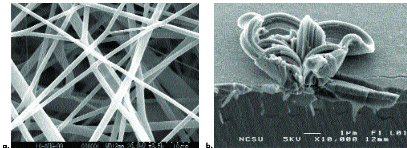
Figure 8. (a) SEM image of a non-woven textile sample of polyethylene oxide fibers. The large depth of field of the SEM makes it possible to image fibers which are 10's of  $\mu\text{m}$ 's below the upper layer of fibers. Bar =  $10\mu\text{m}$ ; (b) SEM image of  $\text{Y}_2\text{O}_3$  crystal. Bar =  $1\mu\text{m}$ .
