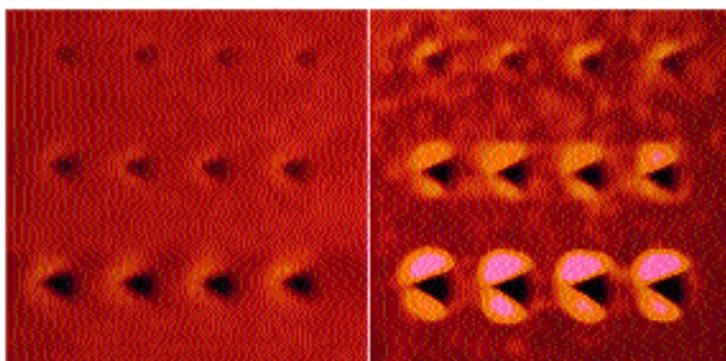
Figure 14. Indentations on two different diamond-like carbon thin films using three different forces (23, 34, and 45 $\mu$ N) with four indents made at each force to compare differences in hardness. 500nm scans.
