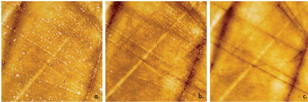
Figure 9. Series of AFM images of the same region on a used RGP lens in saline, (a) before cleaning, (b) after soaking in commercial cleanser, and (c) after soaking in cleanser and rubbing with latex glove. 30µm scans.
