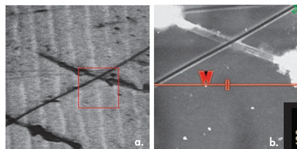
Figure 6. (a) Optical micrograph of a contact lens mold. Approximately 90 x 90μm. (b) AFM top-view image of the same area as box in Figure (a). 20μm scan. (c) AFM cross-sectional plots allow accurate measurements of surface feature height, width, and angle and can be made on any cross-section of the AFM image.
