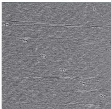
Figure 5. TappingMode AFM image of a hydrogel lens in saline. The grooves of the lens surface are faintly visible and run from lower left to upper right in the image. Periodic defects, running from top left to lower right in the image, are clearly detected. Such defects originate on the diamond-turned mold during the lathing process and are subsequently transferred to the lens surface. 20μm scan.
