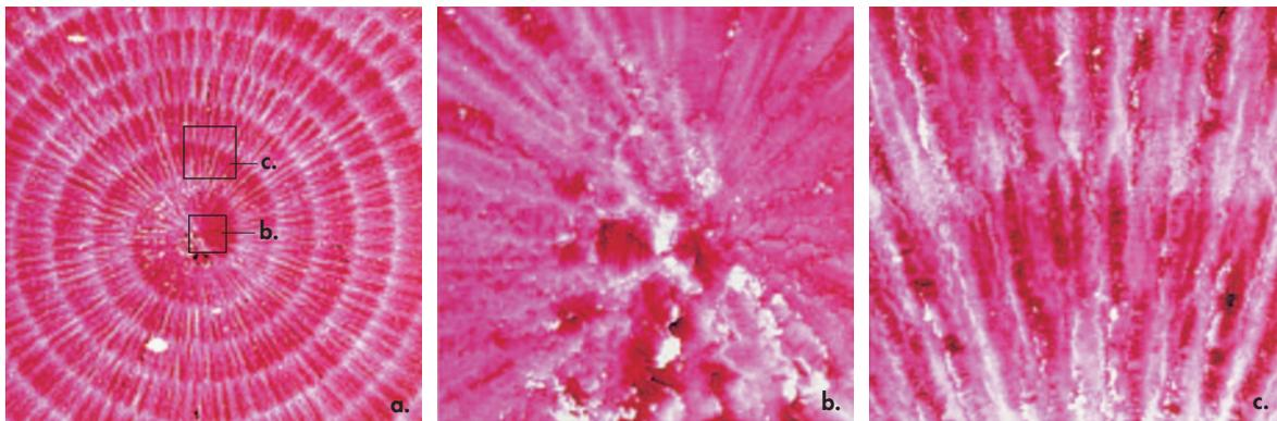
Figure 7. TappingMode AFM image of central area on a diamond-lathed PMMA button (blank). The RMS roughness is 32nm. 50 $\mu$ m scans. Boxed areas in (a) are zoomed and shown in (b) and (c) respectively. Brighter color represents higher features in topography images like these.
