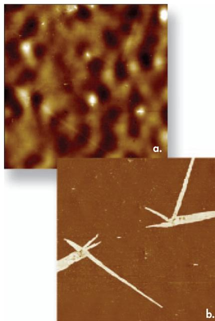
Figure 13. TappingMode topography (a) and phase images (b) of a contact lens in air. Crystalline-like structures in the phase image are possibly salt crystals left after water evaporated from the saline solution. 10 $\mu$ m scans.
