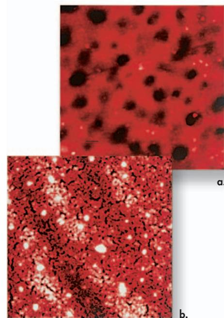
Figure 8. TappingMode AFM images of a (a) hydrophobic silicone hydrogel lens and (b) the same lens material after hydrophilic coating and further processing. Darker areas in (a) are defects that AFM images revealed, and were subsequently eliminated by modifying certain processing steps. 8 $\mu$ m scans.
