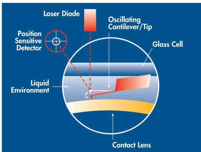
Figure 1. Schematic diagram of TappingMode AFM operation in liquid on a fully hydrated contact lens.
