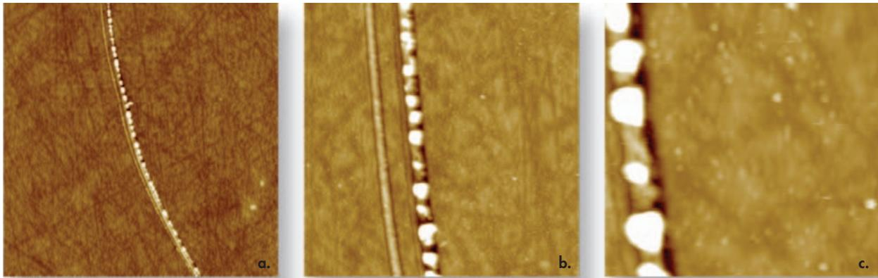
Figure 2. TappingMode in saline solution images of a fresh, out-of-the-box, commercially available contact lens. (a) 47µm, (b) 10µm, (c) 4µm scans.
