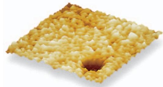
Figure 3. TappingMode image of a 1 $\mu$ m x 1 $\mu$ m area of the same type of contact lens as in Figure 2, also immersed in saline. The RMS roughness is 3.5nm for the area shown. A surface defect or pit, clearly seen in the lower right of the image, measures 170nm in width and 150nm in depth and, therefore, is large enough to trap proteins or contaminants. However, it is too small to be resolved in liquid using conventional techniques.
