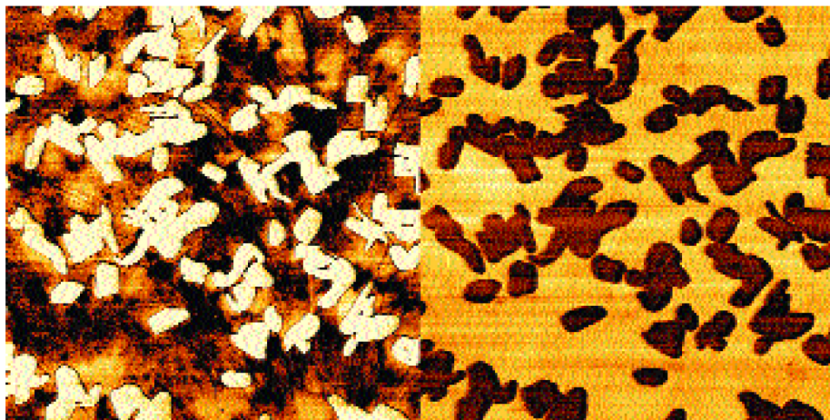
Figure 8. Phase (left) and lateral force (right) images of \text{MoO}_3 crystallites on a \text{MoS}_2 substrate; 6µm scans. The crystallites show light contrast in the phase image, and dark contrast, corresponding to high friction, in the LFM image. Phase gives superior feature detail, and also shows dark regions on the background likely caused by contamination or adsorbed water. Sample provided by Dr. C.M. Lieber, Harvard University.
