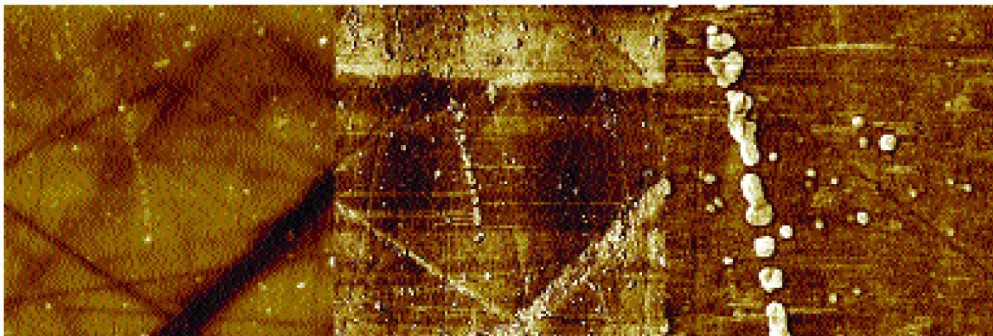
Figure 7. Composite magnetic recording head; 3µm TappingMode and phase images (left and center), and 1 µm phase close-up of contaminants (right). Phase imaging distinguishes the magnetic pole piece (dark) from the gap; the latter appears as a white band across the top of the central phase image. A vertical string of contaminants shows light phase contrast matching that of the gap, suggesting the gap material as the origin of the contamination. Images courtesy Don Chernoff, Advanced Surface Microscopy.
